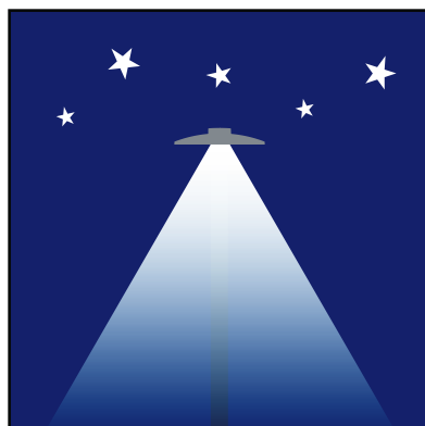
The is a complete cutoff, fully shielded area light that minimizes glare, while reducing light trespass. (The maximum luminous beam angle 90°)
