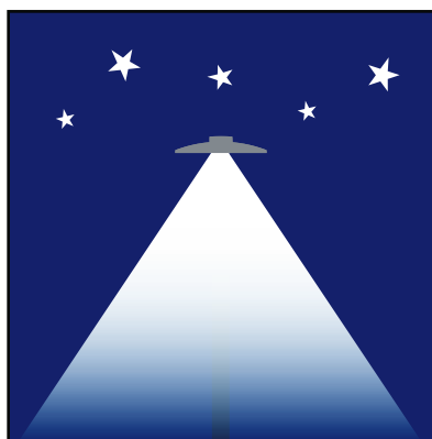
The is a complete cutoff, fully shielded area light that minimizes glare, while reducing light trespass. (The maximum luminous beam angle120°)
